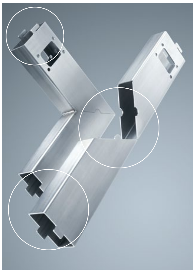
Efficient production of bend connections and positioning aids with a laser.
