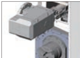
Unloading Unload the finished parts to the Out-conveyor. Side by side : In-conveyor and Out-conveyor.
