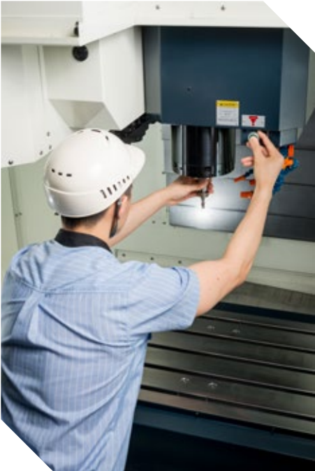
Easy Spindle accessibility for tool loading at spindle side
