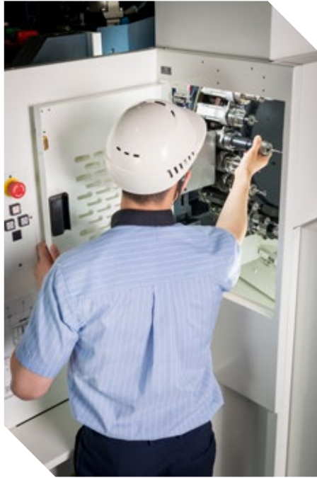
Easy ATC magazine accessibility for tool loading at magazine side
