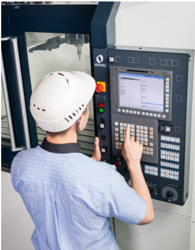
Easy operation with good hand eye co-ordination aided by 90° swing of operation panel
